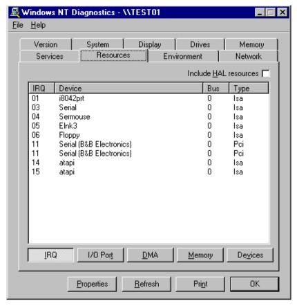
The above shows 2 ports using one PCI card interrupt.
